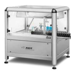
The finite difference method for density measurement relies on the measurement of sample weight dry, and immersed in a fluid, usually water. The difference between the dry and immersed weight is used with the known density of the fluid to calculate the volume of the specimen to a high dvegree of accuracy, irrespective of geometry.
