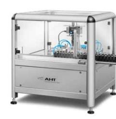
Shore A hardness measurements are based on the precise application of force and the subsequent measurement of probe displacement.
