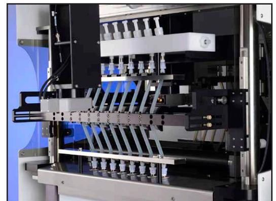
Pulsatile and Axial Distention Synchronized with Rotation and Bending (Proprietary multiaxial loading capability)
