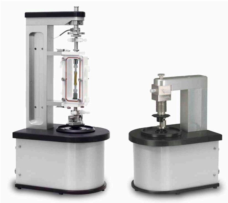
ElectroForce® BioDynamic® instrument with an off-axis pulse can replicate a variety of waveforms
