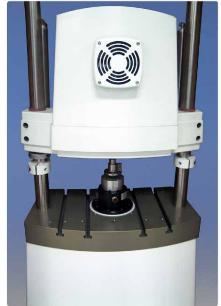
3330 System with Torsion Option and T-slot
