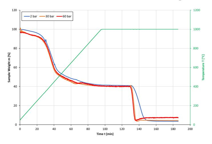
$\frac{dm}{dt} \le 3.0 \%/min$   $\frac{dm}{dt} \le 5.9 \%/min$   $\frac{dm}{dt} \le 5.8 \%/min$   $m_{\infty} = 3.5\%$   $m_{\infty} = 4.4\%$   $m_{\infty} = 7.3\%$
