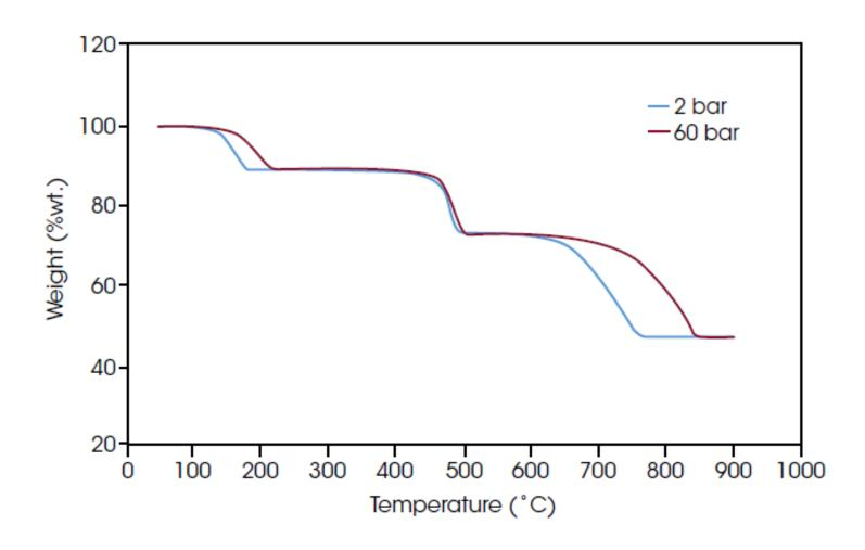
Mass change steps are independent of pressure and can be measured accurately.
