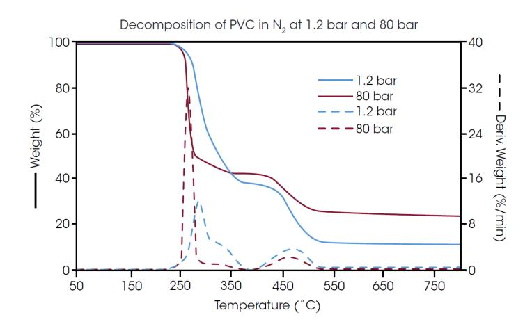
PVC decomposition is a multistage process with HCL and various hydrocarbons as reaction products.
