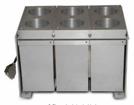
3-Channel calorimeter block
