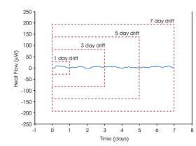
Seven Day Baseline Drift Characteristics for a TAM Air with 3-channel Calorimeter. Red dashed lines represent the baseline drift specification
