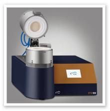
The STA 504 provides simultaneous measurement of weight change (TGA) and heat flow (DSC) on a sample from -160°C to 1650°C. The STA504 features a vertical balance design that is free from errors associated with uncompensated beam growth. DSC heat flow data is dynamically normalized using the instantaneous sample weight at any given temperature.
