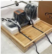
26 Place the ECU box onto the pallet.
