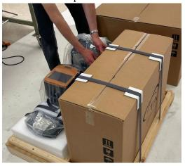
28 The pallet is now ready for the outer box. Place the outer box on the pallet and secure the straps, using the strap protectors as shown.
