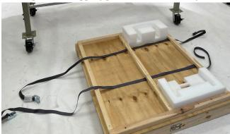
22 Place the bag over the instrument and place the HR into the foam cutout.
