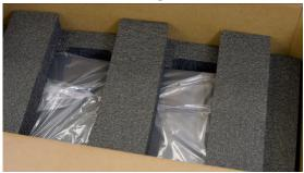
18 Place the inflatable bag inside the accessory cavity of the ECU box.
