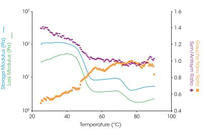
The Rheo-Raman results from the temperature ramp test are shown in the plot above – the data display excellent agreement between bulk rheology and chemical structural changes. As the lotion is heated, the storage and loss moduli drop significantly. This is accompanied by reduction in the Symmetric/Antisymmetric peak ratio and a concurrent increase in the number of Gauche conformers.
