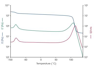
The figure above demonstrates the performance on the DMA mode during a temperature ramp run on an acrylonitrile butadiene styrene (ABS) sample in single cantilever over a temperature range of -100 °C to 140 °C. Two major transitions corresponding to the individual glass transitions of the styrene (-82 °C) and butadiene (115 °C) components are evident, indicating the incompatibility of the two monomers.
