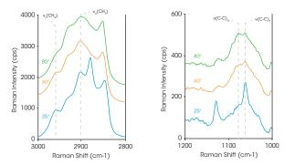
The effect of temperature on the sample spectra is summarized in the plots above. Significant changes were observed in two specific regions of the spectra and the following peaks were identified for further analysis.
