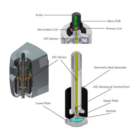
NOTE: Active Temperature Control (ATC) is available for Upper Heated Plate (UHP) and Electrically Heated Plate (EHP) temperature systems.
