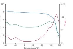
Polymers are often blended to produce a desirable combination of toughness, modulus, and processing characteristics. One such combination is a blend of polycarbonate (PC) with acrylonitrile butadiene styrene (ABS). The ACS-3 provides a sufficient range of temperature control to characterize the multiple low and high temperature transitions of this multi-component sample. The data in the figure were collected during a temperature ramp with a rectangular specimen in torsion.
