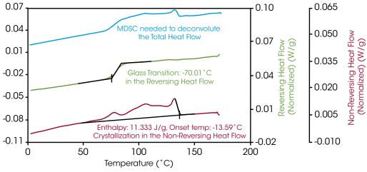
This process oil exhibits a variety of overlapping transitions making interpretation of the Total Heat Flow complicated. On the cooling ramp from 25 to -150°C, MDSC effectively separates crystallization into the Non-Reversing Heat Flow and the glass transition into the Reversing Heat Flow. Gain confidence in data interpretation with the help of MDSC!
