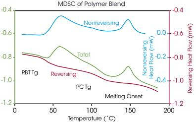
The plot shows MDSC results for a thermoplastic alloy blend of polycarbonate (PC) and polybutylene terephthalate (PBT). This material exhibits a variety of overlapping transitions, and interpretation of the Total Heat Flow is complicated. MDSC effectively separates the crystallization of the PBT component into the Non-Reversing Heat Flow, thereby allowing for accurate determination of the glass transition temperatures of each polymer in the Reversing Heat Flow.
