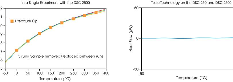
Absolute Zero Heat Flow Baseline Obtained with Tzero Technology on the DSC 250 and DSC 2500
