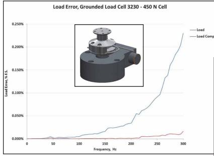
The following is an example of actual improvements through reduction in acceleration induced forces achieved by the ElectroForce<sup>®</sup> Acceleration Compensation Option. The configuration is a ElectroForce 3200 test system with the load cell mounted to the base of the load frame.
