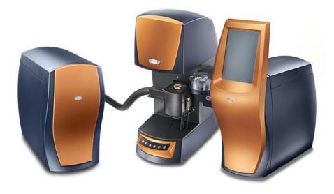
Volatiles from the TGA process are sampled via a heated transfer line into the spectroscopic process.
