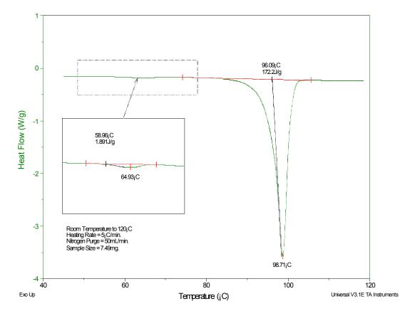
The DSC is an ideal technique for measuring the melting points of crystalline materials and can readily detect multiple crystalline forms when present. The above plot shows a DSC scan run on a crystalline form of sorbitol. This material was run from room temperature to 120 °C at a heating rate of 5 °C/min in a nitrogen purge. Sorbitol can appear in different crystalline forms depending upon the manufacturing process.
