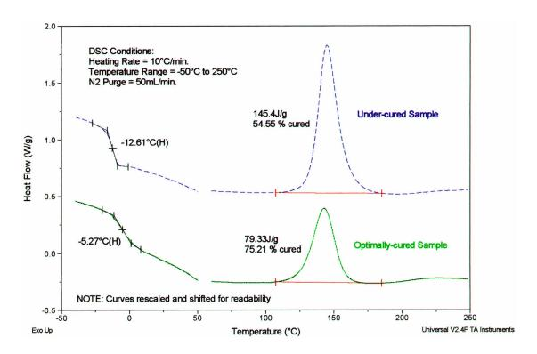
DSC measures the temperatures and heat flows associated with transitions in materials as a function of temperature or time in a controlled atmosphere. This technique provides quantitative and qualitative information about physical and chemical changes that involve endothermic or exothermic processes, or changes in heat capacity.
