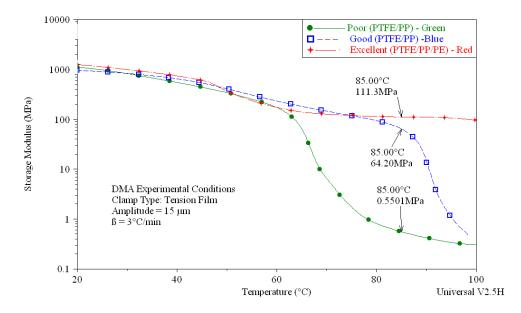
**D**MA measures the modulus (stiffness) and damping (energy dissipation) properties of materials as they are deformed under a periodic stress. These measurements provide quantitative and qualitative information about the performance of materials. DMA is particularly useful for evaluating polymeric materials which exhibit time, frequency, and temperature effects on mechanical properties because of their viscoelastic nature.
