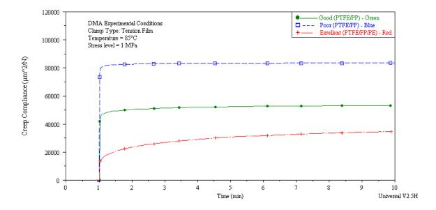
**D**MA measures the modulus (stiffness) and damping, (energy dissipation) properties of materials as they are deformed under a periodic stress. These measurements provide quantitative and qualitative information about the performance of materials. DMA is particularly useful for evaluating polymeric materials which exhibit time, frequency, and temperature effects on mechanical properties because of their viscoelastic nature.
