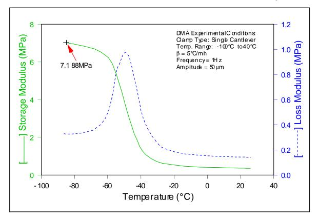
DMA measures the modulus (stiffness) and damping (energy dissipation) properties of materials as the materials are deformed under a periodic stress. These measurements provide quantitative and qualitative information about the performance of materials. DMA is particularly useful for evaluating polymeric materials which exhibit time, frequency, and temperature effects on mechanical properties because of their viscoelastic nature.
