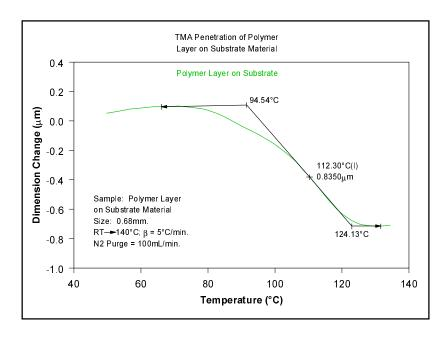
Thermomechanical Analysis (TMA) measures linear or volumetric changes in sample dimension as a function of temperature, time, or force. This data provides valuable information on coefficient of thermal expansion (CTE), penetration, glass transition temperature, softening and flow, and creep/stress relaxation.
