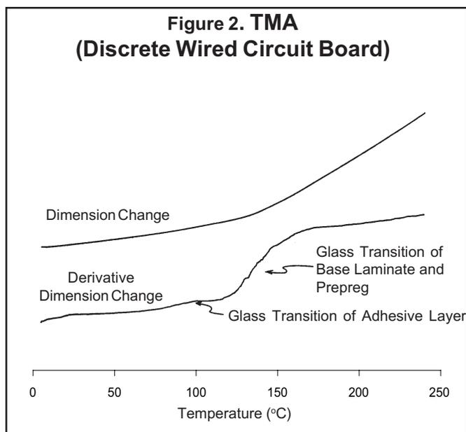
in the expansion coefficient curve. Unfortunately, the TMA Tg's are difficult to quantify precisely by extrapolation from the expansion curve.
