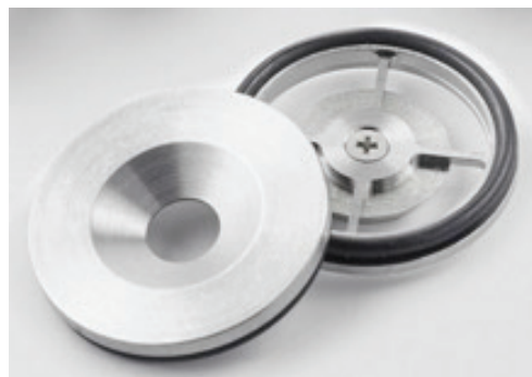
Figure 1. In-Plane fixture for thermal diffusivity analysis of thin samples
