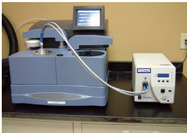
Figure 1: QDSC / PCA System
