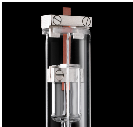
Figure 2. The Film/Fiber Probe loaded with a film in the Discovery TMA 450 RH.
