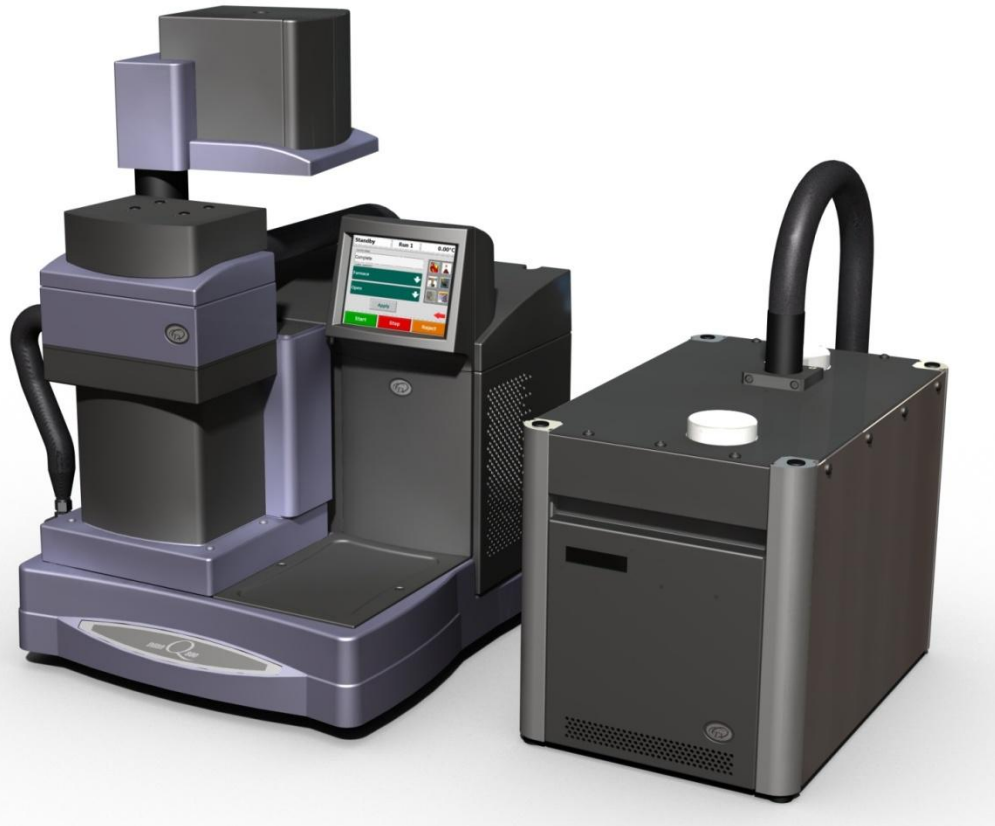
Figure 1: The TA Instruments Q800 Dynamic Mechanical Analyzer with the humidity control accessory
