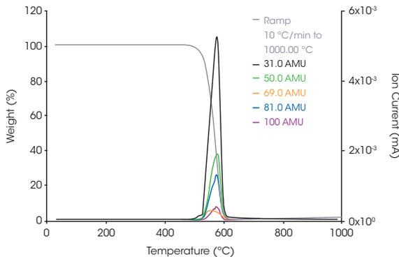
Figure 5. TGA/MS of Polytetrafluorethylene Reference
