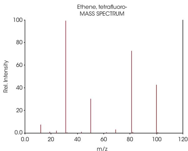
Figure 3. NIST Mass Spec Data Center, S.E. Stein, director, "Mass Spectra" in NIST Chemistry WebBook, NIST Standard Reference Database Number 69, Eds. P.J. Linstrom and W.G. Mallard, National Institute of Standards and Technology, Gaithersburg MD, 20899
