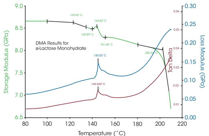
Figure 1:  $\alpha$ -Lactose Monohydrate tested with the powder holder on the DMA. Heating rate 3 °C/min, Test frequency 1 Hz.
