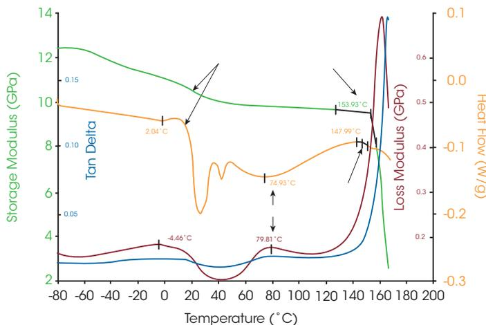
Figure 8: Overlay of the DSC data with the DMA data for the Original Coffeemate
