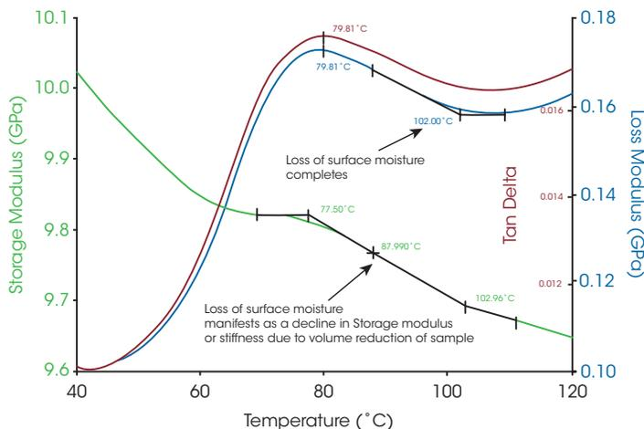
Figure 6: Expanded view of the trace of the Original Coffeemate powder in the region between 40 and 120 °C, where free water loss is expected.
