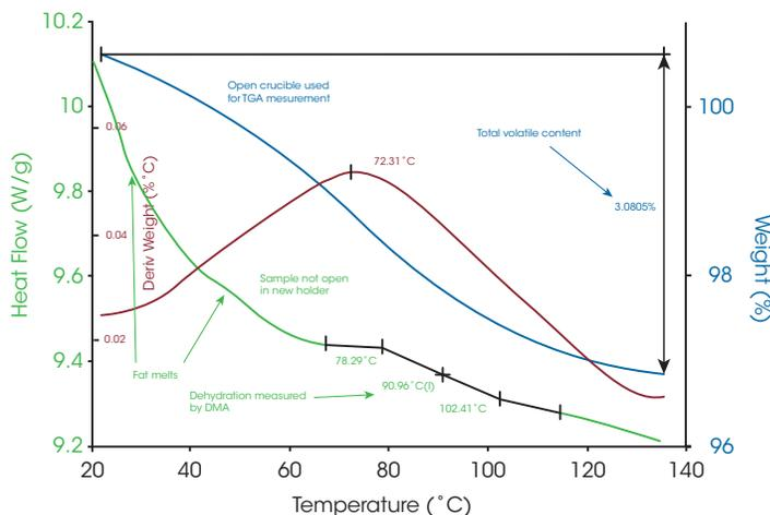
Figure 7: Overlay of the TGA and DMA experiments performed on the Original Coffeemate powder
