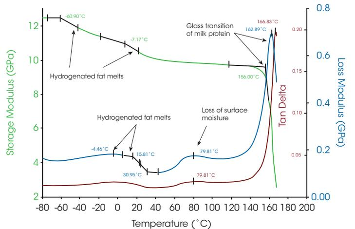
Figure 5: DMA trace of the Original Coffeemate performed at a heating rate of 3 °C/min and a test frequency of 1 Hz.
