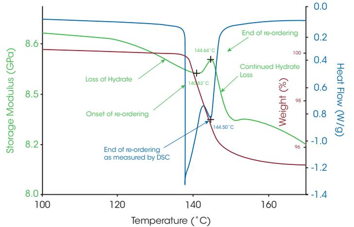
Figure 4: Overlay of DMA, TGA and DSC traces for  $\alpha$ -Lactose Monohydrate.
