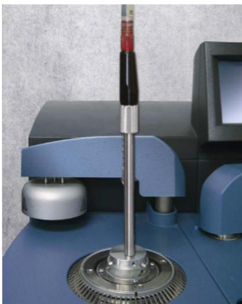
Figure 1. Raman probe interfaced to the Q2000 DSC
