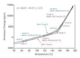
Figure 2: Calculation of CTE, Tg, and Delta Tg from Zone 1 Data
