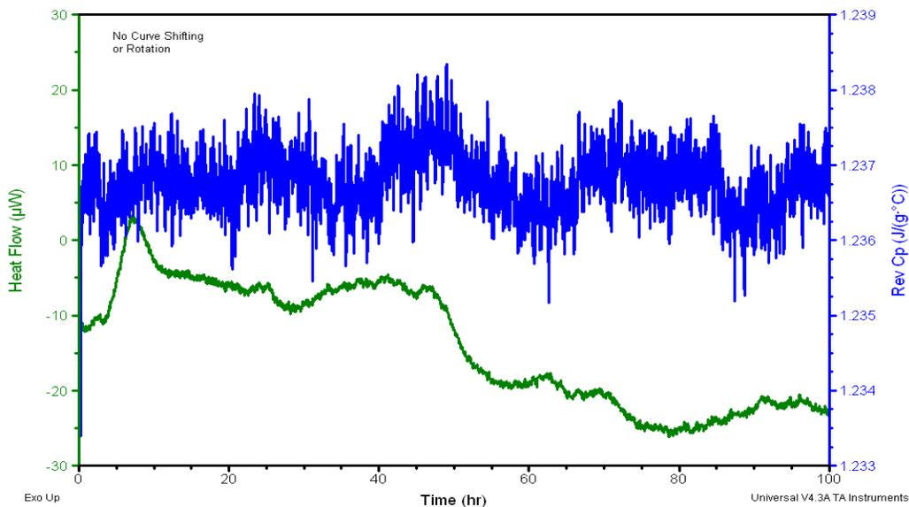
Figure 5. The sensitivity and stability of MDSC are seen in the 100 –hour isothermal data at 50 °C on a 50/50 mixture of acetylsalicylic acid (Aspirin) and crystalline sucrose
