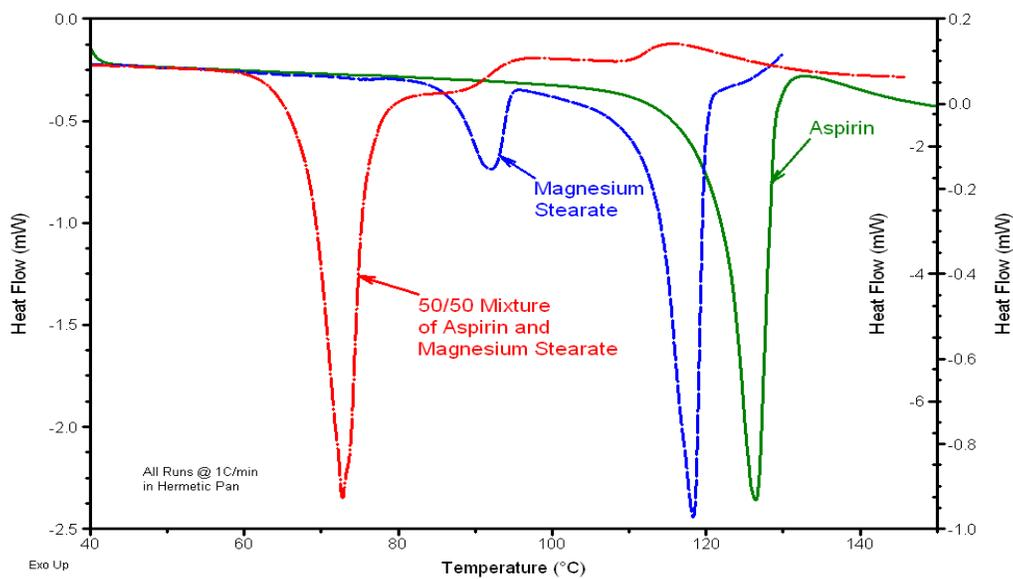
**Figure 3.** Comparative DSC results on the drug, excipient and 50/50 mixture at a heating rate of 1 °C/min. Results indicate strong interaction between aspirin and magnesium stearate
