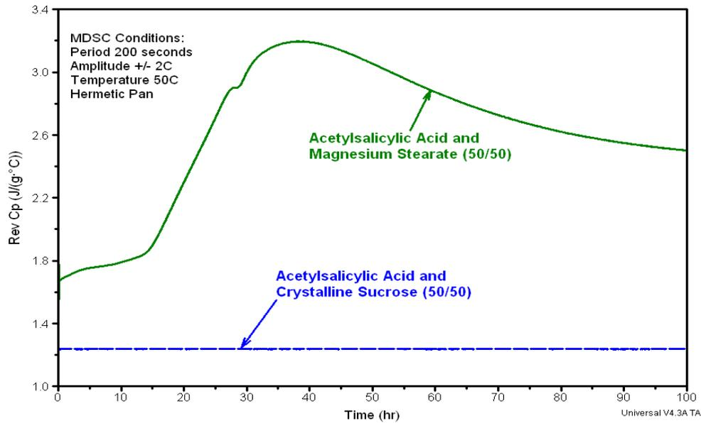
**Figure 6. A comparison of the MDSC® Reversing Cp signals from the 100-hour, 50 °C isothermal experiments show that acetylsalicylic acid interacts with magnesium stearate but not sucrose**
