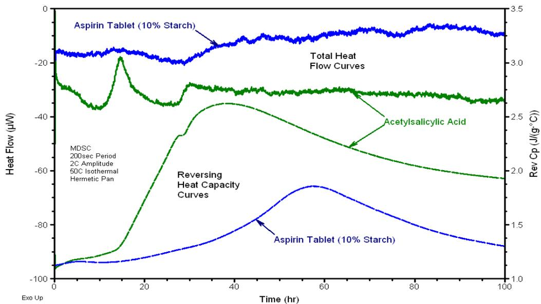
Figure 4. The Reversing Cp signal shows strong interaction between aspirin and magnesium stearate even at 50 °C. The rate of reaction is too slow to be measured by the heat flow rate
