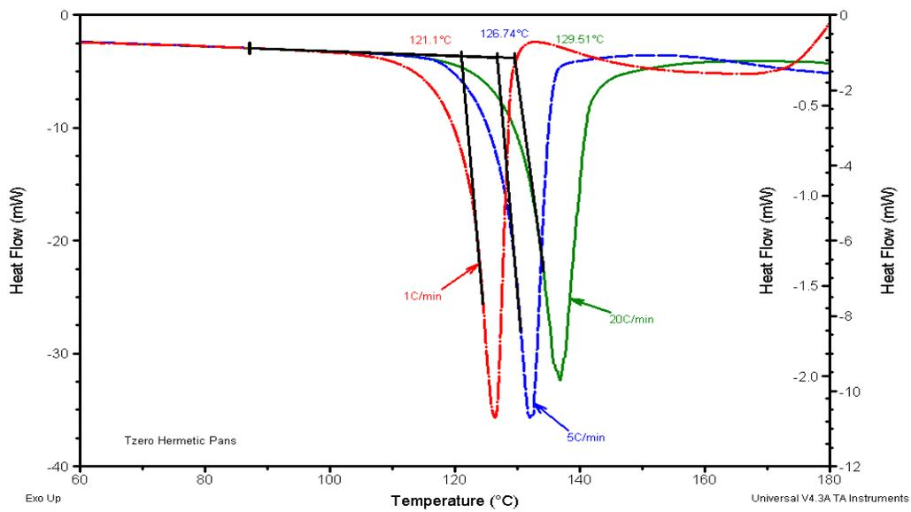
**Figure 2.** The effect of heating rate on the apparent melting point of an aspirin tablet (Acetylsalicylic acid with 10% starch). The temperature shift indicates decomposition
