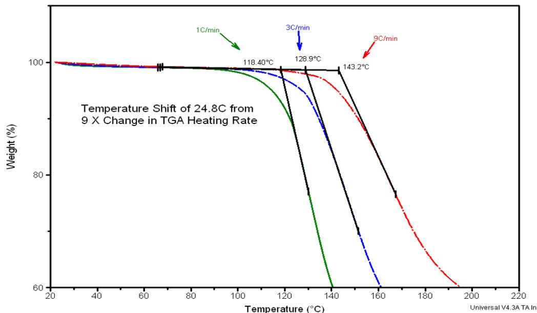
**Figure 1. The effect of heating rate on the temperature of decomposition for an aspirin tablet**
