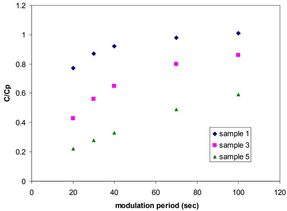
Figure 1 – Ratio of the Apparent heat Capacity © to the Specific Heat capacity (C<sub>p</sub>) Versus Modulation Period for Different Samples
