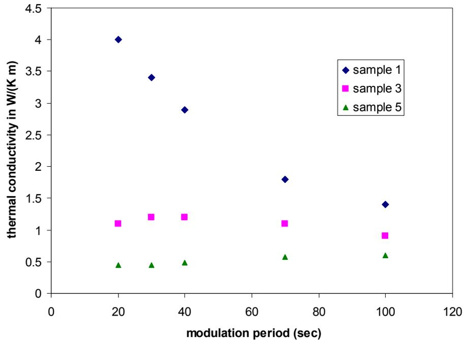
Figure 2 – Thermal Conductivity Versus Modulation Period for Different Samples
