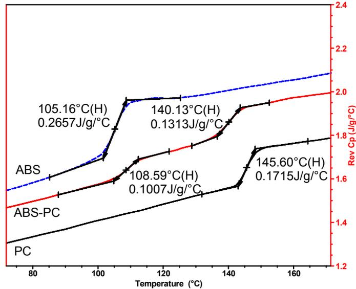
Figure 6 – Reversing Heat Capacity for PC, ABS and PC-ABS Alloy
