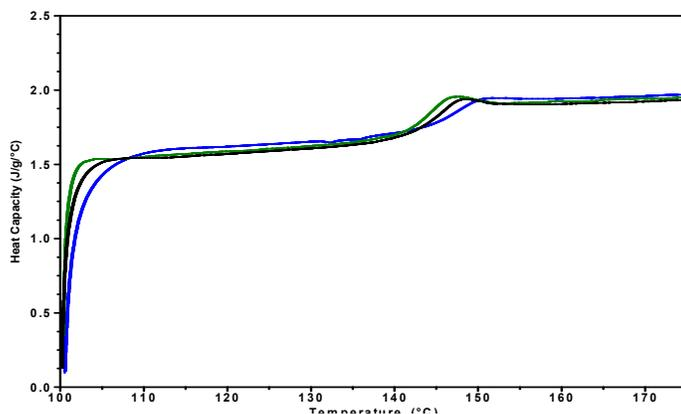
Figure 3 – Polycarbonate Heat Capacity at 5, 10 and 20 °C/min
