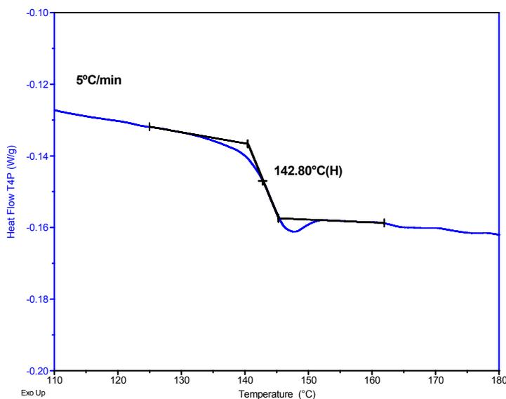
Figure 1 – Glass Transition of Polycarbonate
