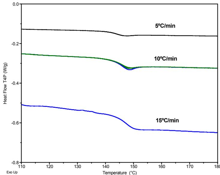
Figure 2 – The Glass Transition of Polycarbonate at Three Heating Rates. The 10 °C/min Data is from Three Samples Cooled at 5, 10 and 20 °C/min.
