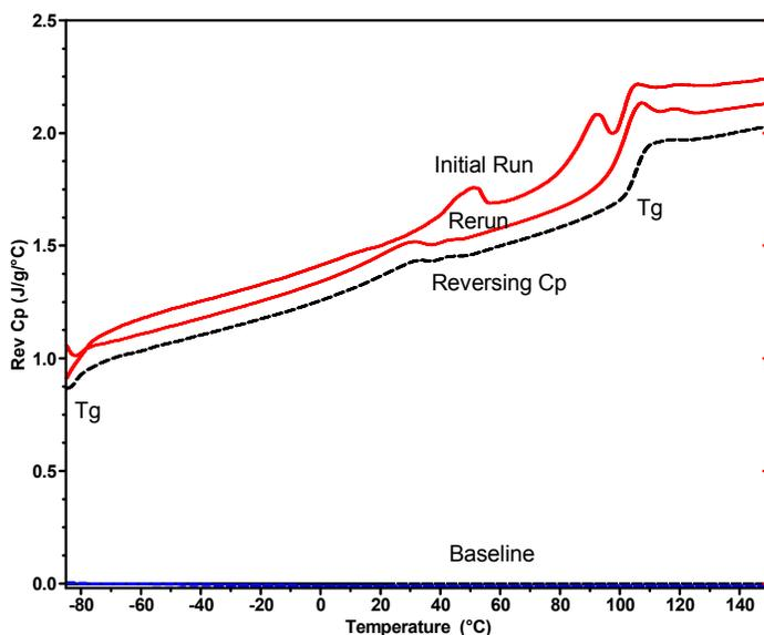
Figure 4 – Heat Capacity of ABS, Initial Heat, Reheat and Reheat Reversing Signal
