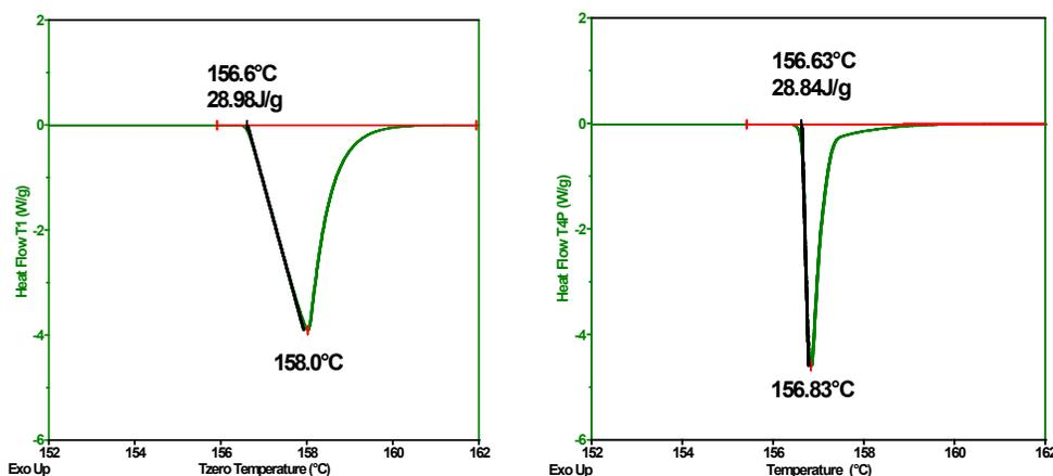
Figure 3 - 3.5 mg Indium by Traditional DSC (left) and Using Advanced Tzero™
