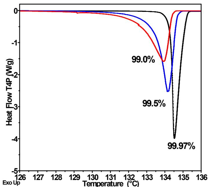
Figure 1 - DSC Melting Curves of Phenacetin at Three Purity Levels
