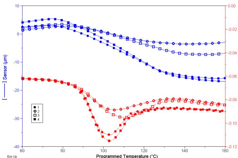
*Figure 3. Localised Thermal Analysis data from 4 locations across a Polyethylene Gel Particle.*
