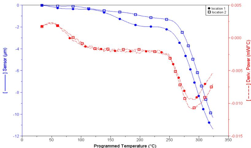
Figure 1. Localised Thermal Analysis data from two locations on a Nylon 6/6 pellet.
