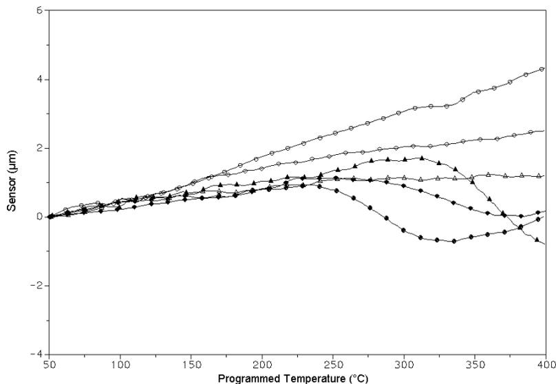
Figure 6. Micro-Thermomechanical Analysis data obtained from the surface of a polymer weld.
