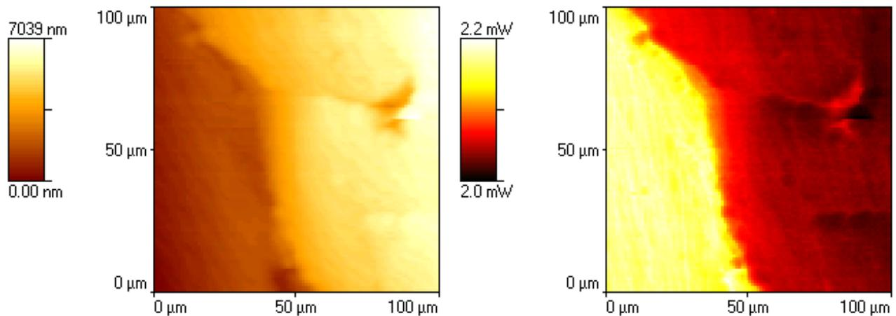
*Figure 4. Topography (left) and Thermal Conductivity (right) images of a heater wire embedded in a polymer substrate.*
