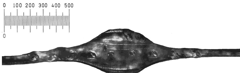
*Figure 2. Optical Micrograph of a Gel Particle cut from a Polyethylene Film*
