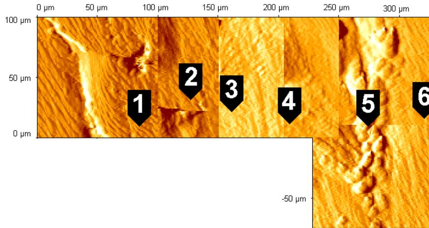
Figure 5. Composite Topography image of the polymer weld showing the locations of the Local Thermal Analysis experiments.
