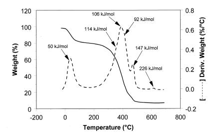
Figure 1 shows the weight loss and rate of weight loss profiles for a coal sample. The volatile carbon weight loss between 300 and 500 °C with peaks in the derivative curve seen at 374, 447 and 580 °C and shoulders or inflections at 325 and 391 °C. The MTGA generated continuous activation energy may be marked for any point in the weight loss region. The determined activation energy is that for the mix of reactions occurring at the particular temperature and conversion.
