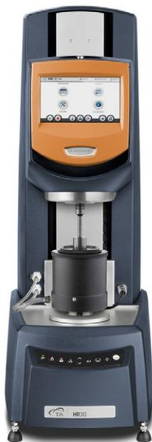
Figure 2. Concentric Cylinder configuration on a TA Instruments Discovery HR-30 Rheometer
