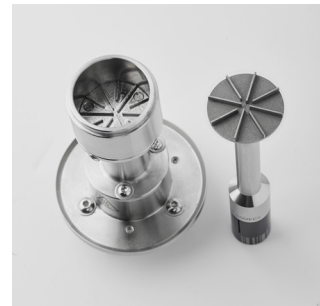
Figure 1. Discovery HR Rheometer with Powder Rheology Accessory shear cell
