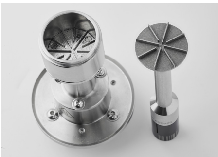
Figure 3. Shear cell serrated upper plate and cup
