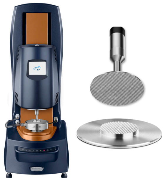
Figure 1. DHR-2 rheometer (TA Instruments) with crosshatched plate-plate 25 mm geometry used to determine the viscoelastic properties of collagen hydrogels.
