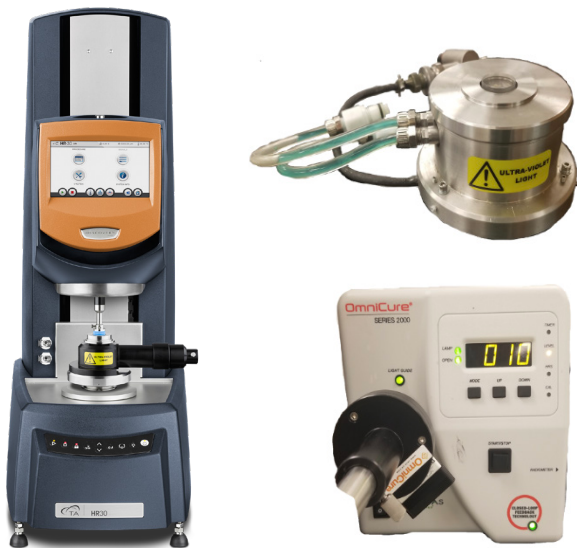
Figure 2. (Left) Picture of TA Instruments HR-30 Rheometer equipped with the light guide UV geometry. (Upper Right) Image of the single wavelength LED UV fixture (available in multiple wavelengths). (Bottom Right) The OmniCure source unit provides a spectrum of wavelengths using a mercury lamp to the light guide fixture (available with optical filters for specific wavelengths).
