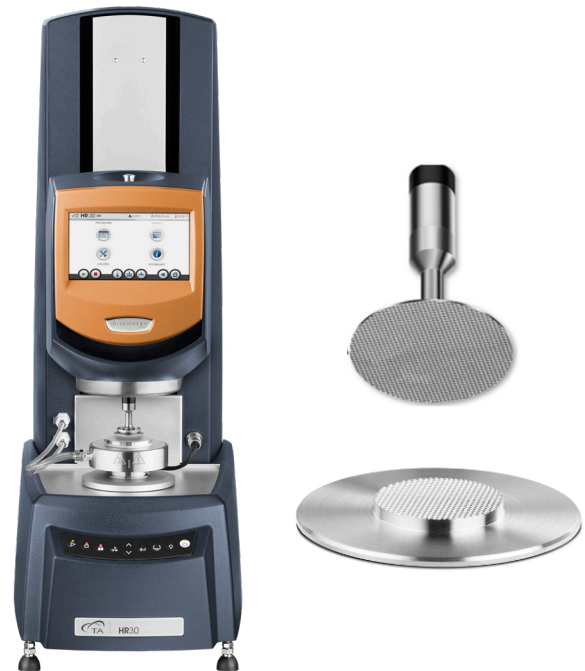
Figure 1. Picture of TA Discovery HR-30 rheometer with a crosshatched parallel plate geometry
