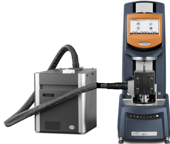
Figure 1. TA Instruments Discovery Hybrid Rheometer with the relative humidity accessory
