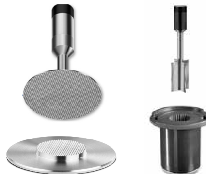
Figure 1. Rheometer accessory setup with roughened geometry, vane rotor, and grooved cup
