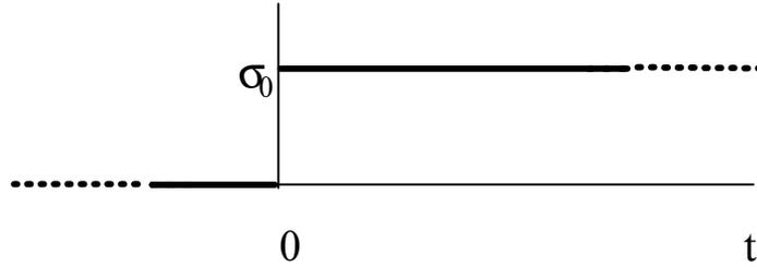
Figure 1: Stress history for a standard creep test
