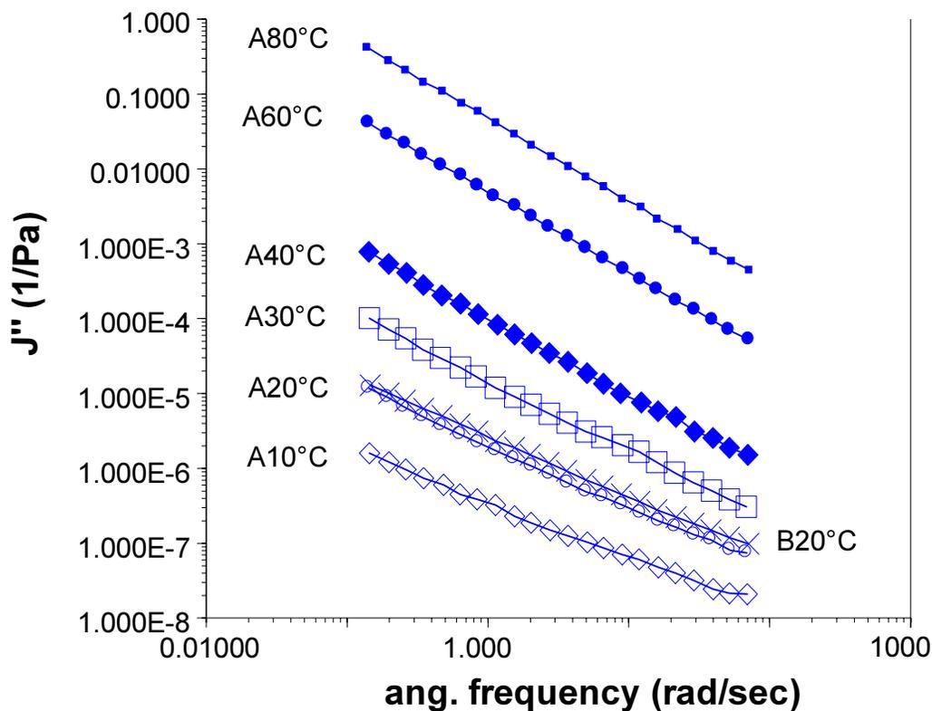
Figure 4: Loss compliance,  $J''$ , against angular frequency,  $\omega$ , for Samples A and B at all temperatures. Crosses indicate Sample B
