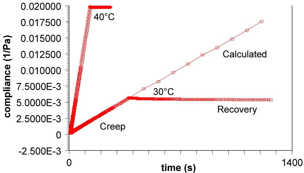
Figure 6: Creep compliance,  $J(t)$  against time for Sample A at 40°C and 30°C, showing creep, recovery and calculated parts of curve.
