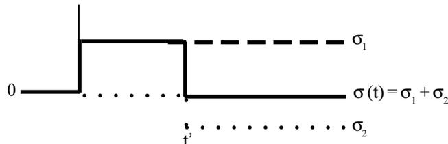
Figure 2: Stress history for creep test with stress removed at time  $t'$ .
