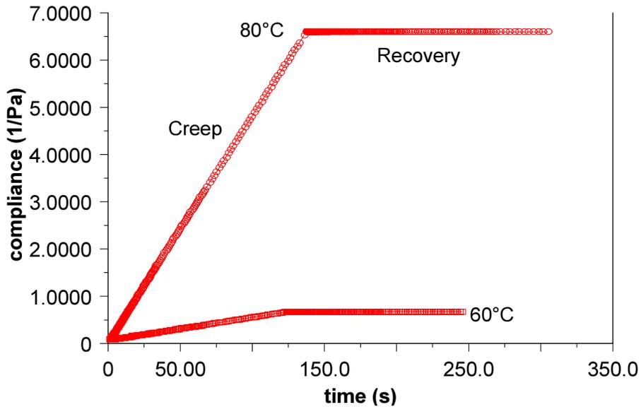
Figure 5: Creep compliance,  $J(t)$ , against time for Sample A at 80°C and 60°C, showing creep and recovery parts of curve.
