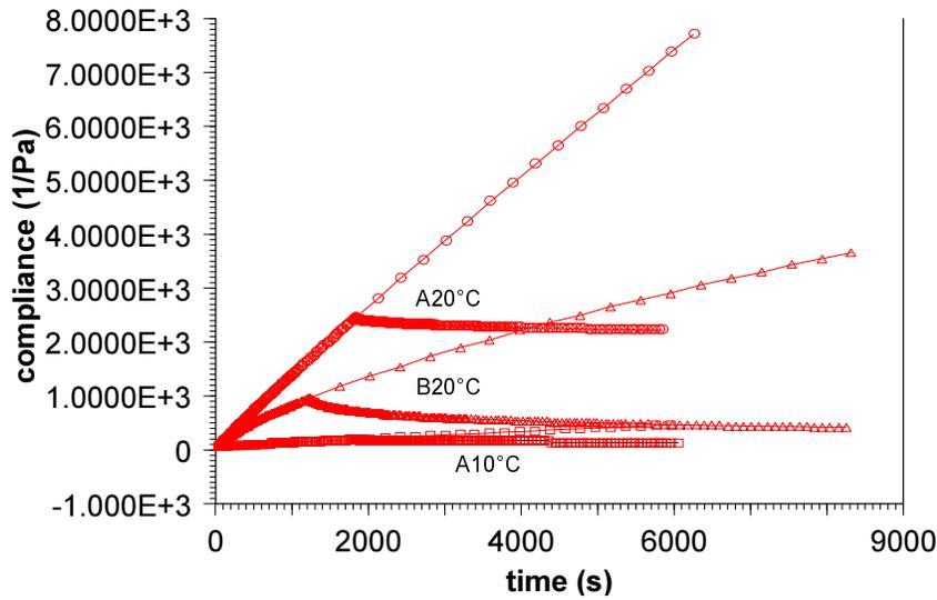
Figure 7: Creep compliance,  $J(t)$ , against time for Sample A at 20°C and 10°C and Sample B at 20°C, showing creep, recovery and calculated parts of curve.
