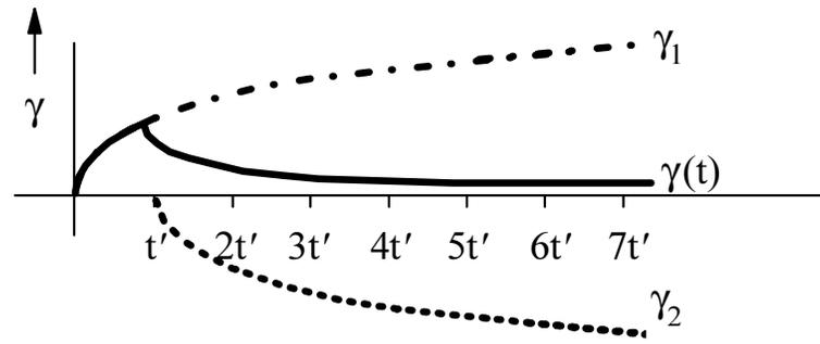
Figure 3: Strain response to incomplete creep test
