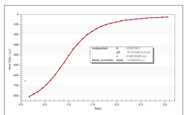
Figure 4. Binding analysis of (NAG) $_3$  to Lysozyme using Incremental Injection ITC: The area under each peak integrated and fit to a one-site Independent binding model and a Blank (constant) (red) to determine the binding affinity (K) 3.23 x 10 $^4$ , enthalpy (dH) -37.91 kJ/mol and stoichiometry (n) 0.995 mol. The heat of dilution was subtracted from the integrated peak area and is represented by the Blank (constant) (blank) -4.08  $\mu$ J.
