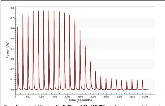
Figure 1. Incremental titration of 1mM HCl into 0.18 mM KHCO<sub>3</sub>: Each peak corresponds to a single titration of HCl into a solution of KHCO<sub>3</sub> at specific time intervals. The titration data is measured in  $\mu$ W.
