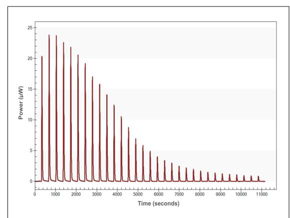
Figure 3. Binding analysis of (NAG) $_3$  to Lysozyme using Incremental Injection ITC: Raw incremental-titration data plotted as power ( $\mu$ W) versus time (sec). Each peak corresponds to injection of NAG $_3$  into the lysozyme solution
