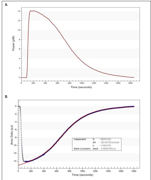
Figure 4. Binding analysis of (NAG)<sub>3</sub> to Lysozyme using Continuous Injection ITC: A. Raw continuous-titration data in  $\mu$ W. B. The points were then fit to a one-site Independent binding model and a Blank (constant) (Red) was used to determine the binding affinity (K) 3.51 x 10<sup>4</sup>, enthalpy (dH) -36.45 kJ/mol and stoichiometry (n) 1.04 mol. The Blank (constant) value subtracted from each data point was -0.96  $\mu$ J.
