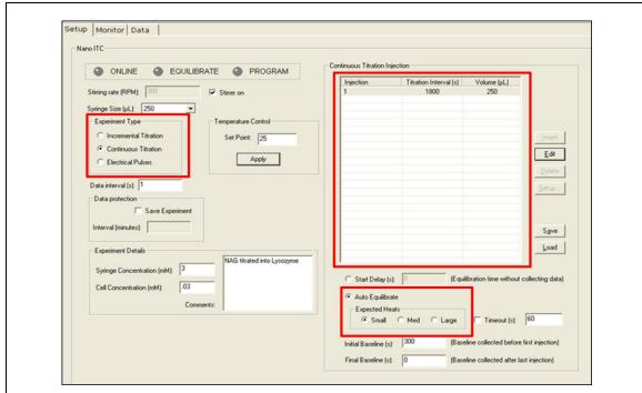
**Figure 2. Continuous-ITC Experiment Setup:** "Continuous Titration" Experiment Type was selected (red box, left) and then the Continuous Titration Injection parameters set (red box, right). Auto Equilibrate function (red box, bottom) has three settings pertaining to the Expected Heat (Small, Medium and Large) for each injection.
