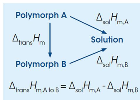
Amplitude calorimetry can be used to study the kinetics of transition of one form into another in terms of the heat flow as a function of time. Transformation of a meta-stable form into the
