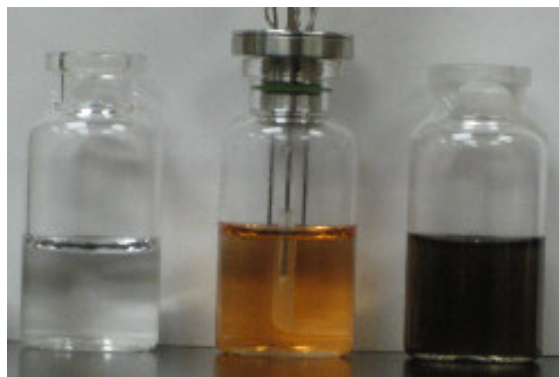
Figure 3: Left - blank experiment with ambient air, Middle - nitrogen purged, Right - ambient air
