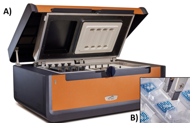
Figure 1. A) TA Instruments RS-DSC and B) disposable microfluidic chip (MFC) and cover slip.
