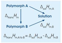
Ampoule calorimetry can be used to study the kinetics of transition of one form into another in terms of the heat flow as a function of time. Transformation of a meta-stable form into the
