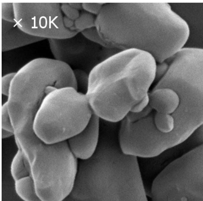
**Figure 3A.** An SEM of micronised sucrose stored at room temperature.
