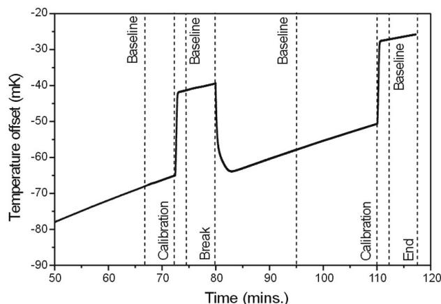
**Figure 1.** A typical example of the response from the SolCal, in this example, as received  $\alpha$ -lactose monohydrate.
