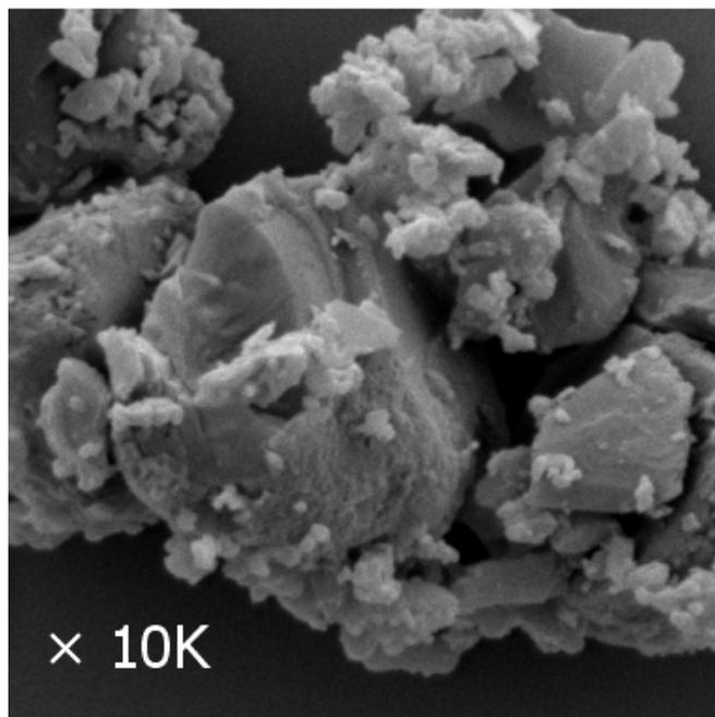
**Figure 3B.** An SEM of micronised sucrose stored in a freezer.
