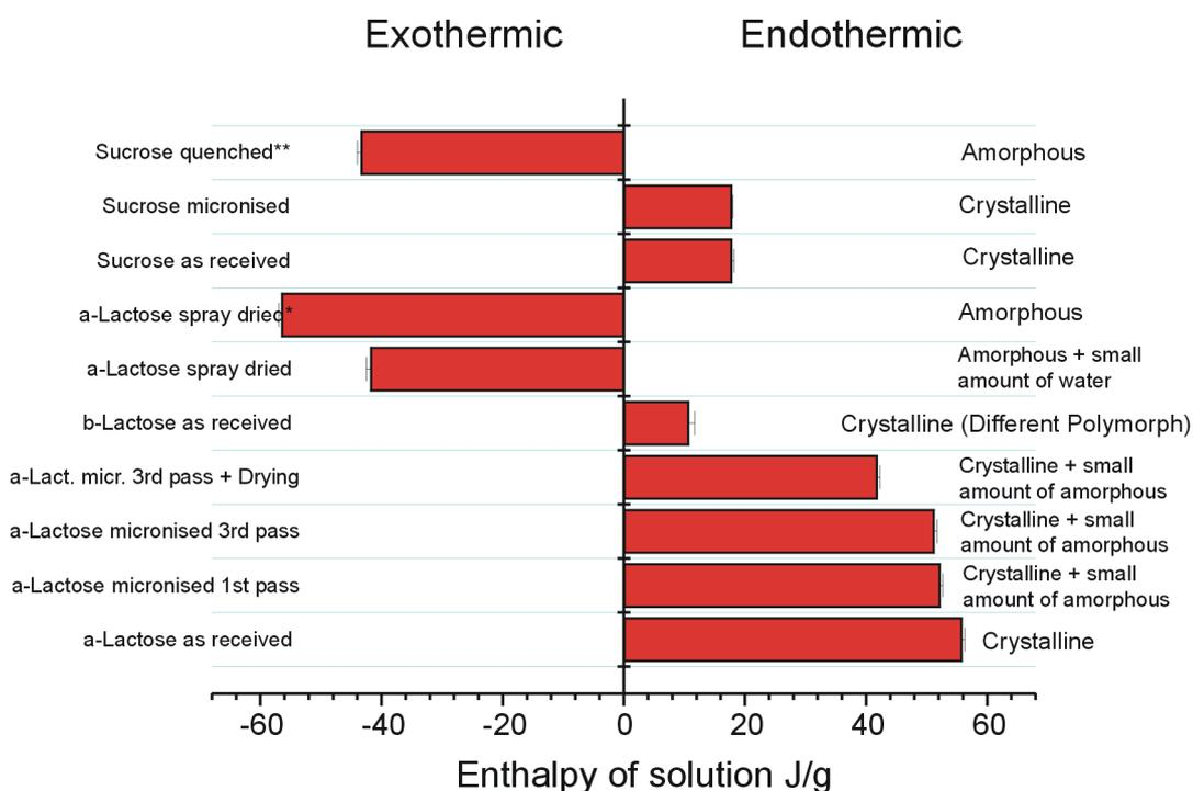
**Figure 2.** A summary of the enthalpies of solution at 25°C in water for lactose and sucrose processed and stored under different conditions. Each bar represents the average of three experiments (average standard error = 0.5 J/g).
