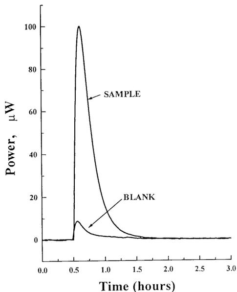
**Figure 1.** A typical calorimetric response to the adsorption of water vapor on sodium benzoate at 25°C. Sample size 100 mg, relative humidity 10%, total flow rate 2.0 mL/min (0.2 mL/min water saturated nitrogen and 1.8 mL/min dry gas).
