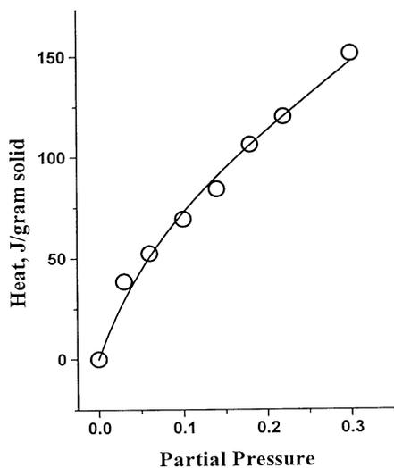
**Figure 3.** The calorimetric adsorption isotherm of water vapor on sodium benzoate at 25°C. Each point represents an average of three replicates. The curve is the least squares generated using Equation 1.
