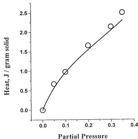
**Figure 4.** Water sorption isotherm derived calorimetrically for an amorphous solid decapeptide at 25°C. The symbols are experimental points and the line least squares generated using Equation 1.
