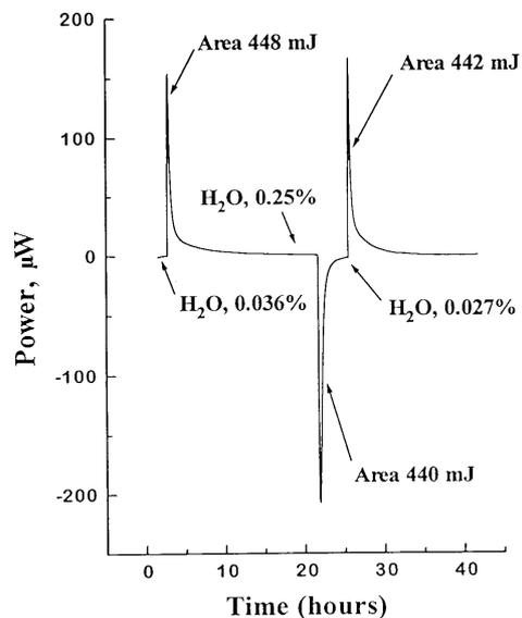
**Figure 2.** Adsorption-Desorption cycles of water on sodium benzoate at 25°C and 40% relative humidity. The water content at the beginning and the end of the experiment are also shown.
