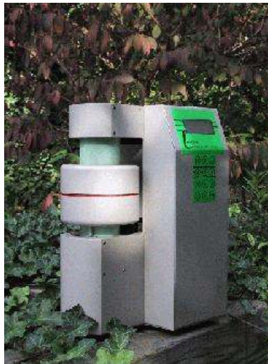
Figure 1. FOX50 Heat Flow Meter Instrument, LaserComp, Inc.
